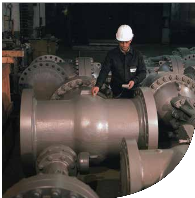
PAINTING CONTROL - PAINTING THICKNESS CHECK
