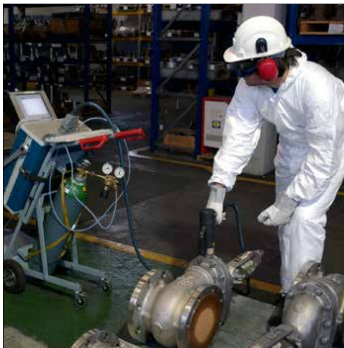
CHEMICAL ANALYSIS, SPECTROMETER P.M.I. POSITIVE MATERIAL IDENTIFICATION
