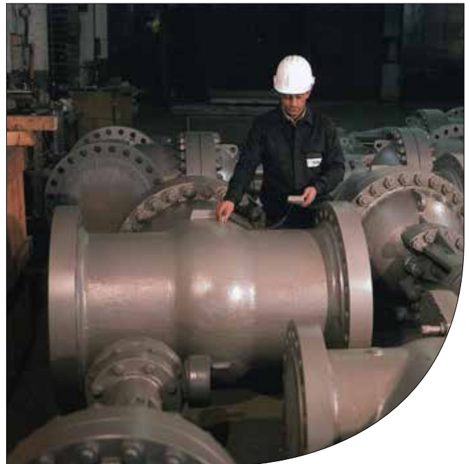
PAINTING CONTROL - PAINTING THICKNESS CHECK
